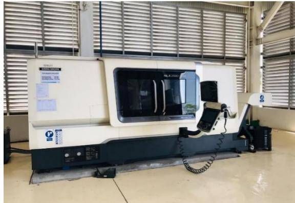
CNC Lathe Machine Type NLX 2500 Y / 1250
